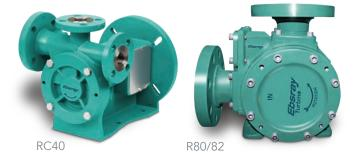
periphery. As liquid enters the suction port, kinetic energy carries it around the narrow hydraulic channel around the cells, creating the energy and differential pressure that moves the liquid through the pump. Other advantages of Ebsray pumps include a small footprint, high efficiency that requires smaller motors, quiet operation with no vibration and easy maintenance.
