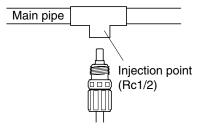
(2) Wind sealing tape around the external thread of the anti-siphon check valve, and screw the valve into the injection point.
