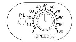
Adjustable range of stroke speed: 15 to 300 strokes/min
