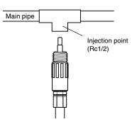
(2) Wind sealing tape around the external thread of the anti-siphon check valve, and screw the valve into the injection point.
