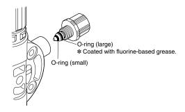
(3) Hold the retaining nut (the part shown by the arrow), turn it clockwise, and install it on the pump head.
