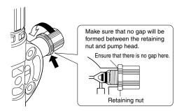
(4) After installing the relief valve, rotate the air-release knob by two turns in the clockwise direction to ensure that the O-ring is seated properly.
