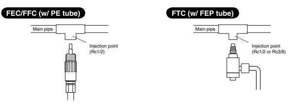
(2) Wind sealing tape around the external thread of the anti-siphon check valve, and screw the valve into the injection point.
