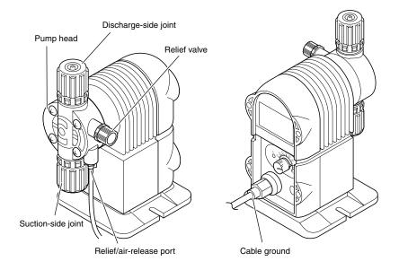
\* The shapes of pump heads and joints differ slightly depending on the liquid-end material and connection type.
