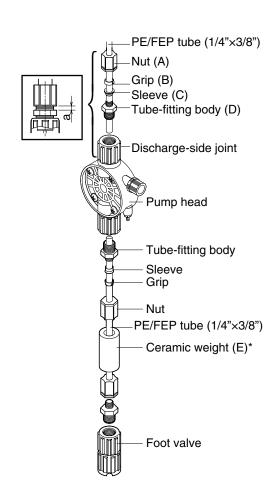
\* The tube is packed in the form of a coil. Attach the ceramic weight (E) and straighten out the tube so that the liquid inside the tank will be sucked up through it.
