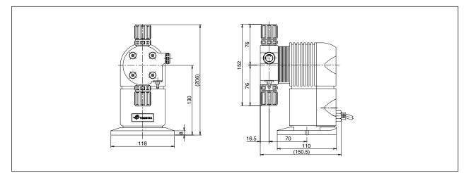
Model w/ automatic air-release function for injection of sodium hypochlorite: ARPZ-31/61/12
