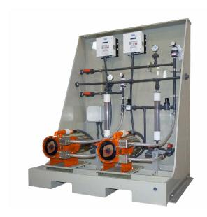
A wastewater-treatment plant's chemical-transfer system can be optimized through the use of peristaltic pumps because the technology does not contain any valves that can become clogged. This means that when the pump is shut down any viscous liquids that will generally solidify or become gelatinous when resting will not adversely affect the pump's operational capabilities.
