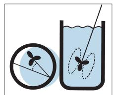
FIGURE 1 - Angling the portable mixer off-center is the position recommended by Neptune for rapid turnover of tank contents and good bottom washing.
