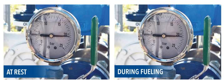
*Ebsray®* Regenerative Turbine Pumps excel in the transfer of Autogas because they can create more than enough differential pressure between the storage tank and the vehicle's fuel tank. At rest, an LPG storage tank can typically have a pressure of 8 bar (116 psi), left photo, but when fueling begins the Ebsray pump can create 21 bar (305 psi), which is more than enough to facilitate the fueling process.
